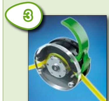
3 Open up the lever and fit the claw over the other set of dowels
