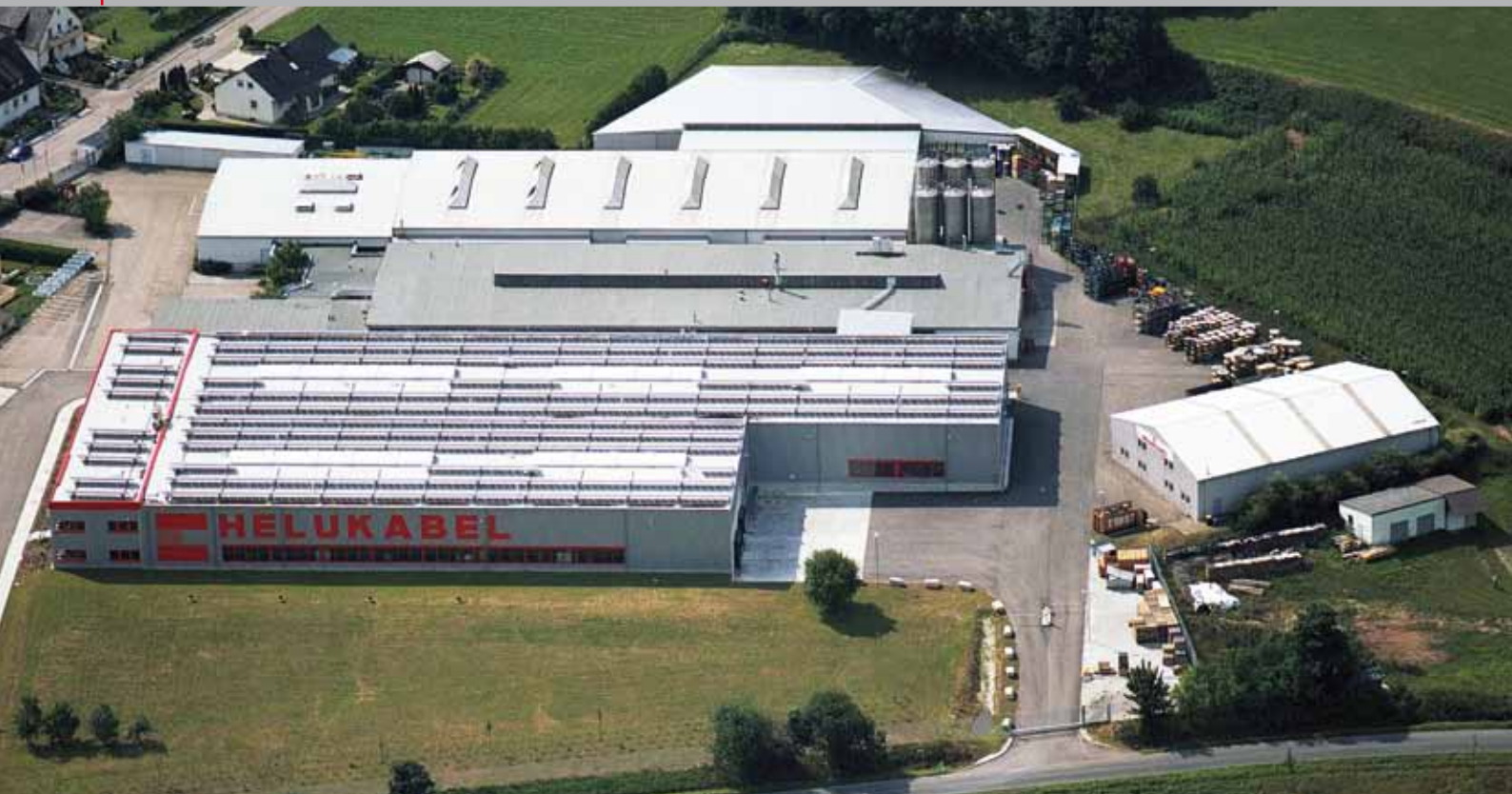
Photo: Our production in the Windsbach plant with a modern photovoltaic system with 1125 solar modules. The system provides an annual energy amount of 970 kWh per KWp = 185,512 kWh. This saves our environment approx. 111 tons of CO 2 per year.
