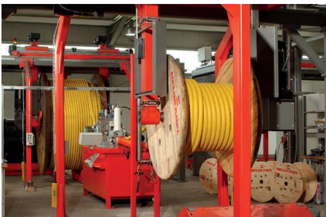
Heavy-load length-cutting facility
