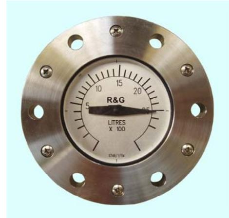
Bayham direct reading tank contents gauges are designed for mounting directly onto the side of a tank to provide a continuous reading of product contents. Each gauge incorporates a magnetic coupling through the gauge body from the wet side to the pointer, which eliminates the possibility of fluid leakage into the gauge dial chamber. The dial chamber is completely sealed and is supplied with a dry nitrogen purge to prevent condensation or ice formation under low operational temperatures.
